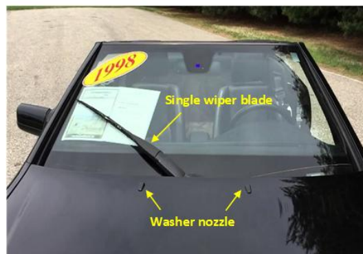
Fig. 9. Mono wiper blade of Mercedes-Benz W124 [10]
