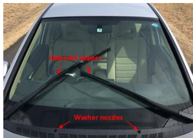
Fig. 16. Opposed pattern wiper blade of Honda Civic [16]
