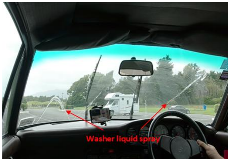
Fig. 8. Narrow blade spacing of Porsche 911 [9]
