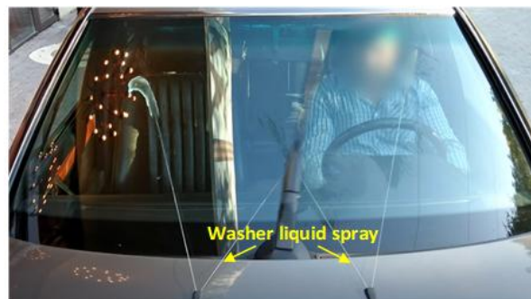
Fig. 10. Washer nozzle function of Mercedes-Benz W124 [11]
