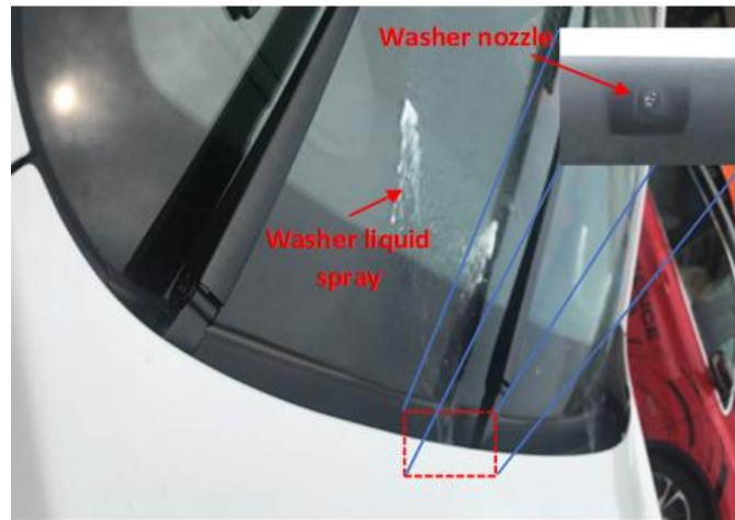
Fig. 18. Washer liquid dispensing from Proton X70
