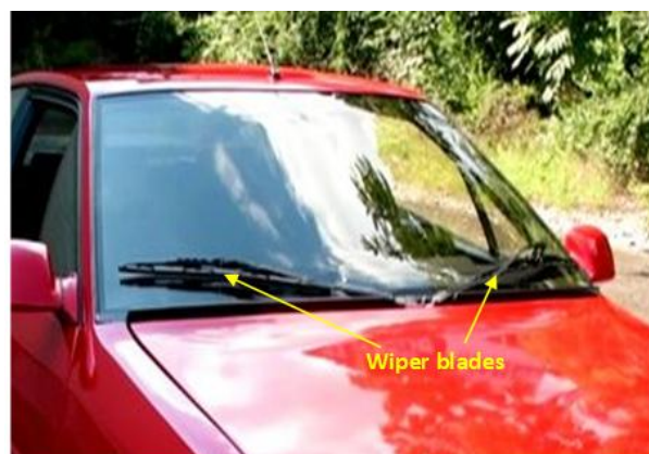
Fig. 5. Opposed wiper system of Alpine A310 [8]
