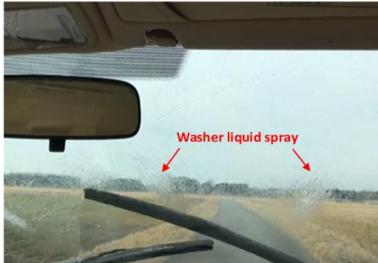
Fig. 17. Spray of washer liquid on Honda Civic [16]
