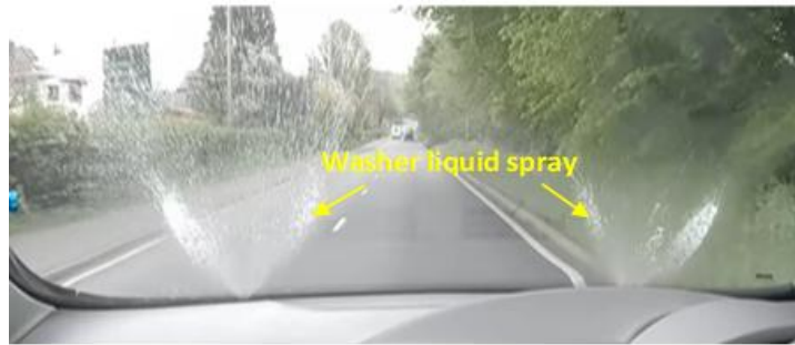
Fig. 15. Spray of washer liquid on SEAT Altea [15]
