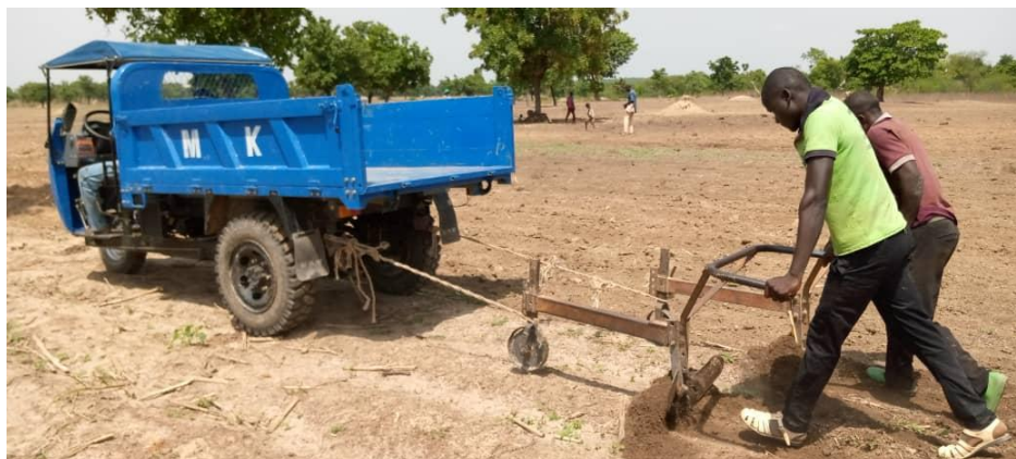
Picture 1. Motorized plow with a trike used for tilling
