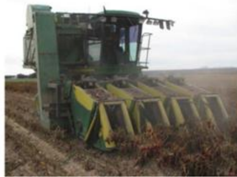
Fig. 2. McClendon four-row self-extracting dry red pepper harvester
