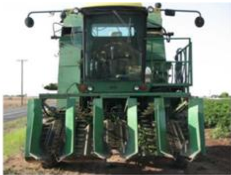
Fig. 1. Massey's three-row self-propelled pepper harvester
