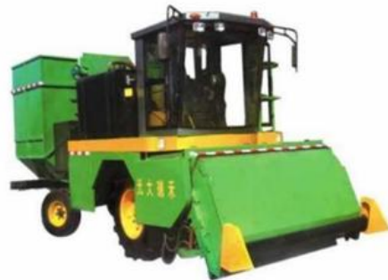
Fig. 3. 4JZ-3.6 self-propelled pepper harvester
