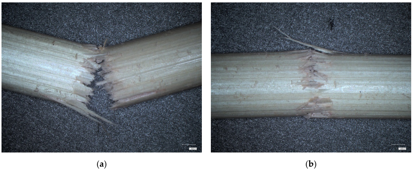
Figure 9. Partially cut straw. (a) Detail of the cut region. (b) Detail of the uncut region.
