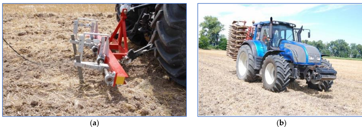
Figure 3. Field measurements. (a) Depth of the horizontal penetrometer blades (field measurement). (b) Valtra T202 tractor with Kverneland Qalidisc discs (Kverneland Group, Klepp, Norway).
